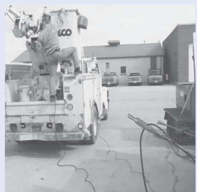
A Delta technician attaches a test lead to one of the bucket areas of the truck.
